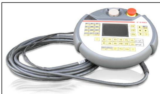
Easy handling of the FMB loading magazine is supported by a detachable user-friendly control panel. It can be combined with a high-performance programmable logic control (PLC) system to enable FMB to produce very flexible customer-specific special functions and processes.
